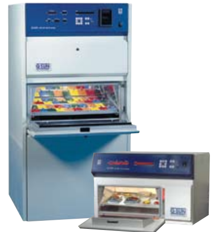
Q-Sun models range from an entry level, bench-top model to a full-featured tester with humidity control, water spray, and chiller.
