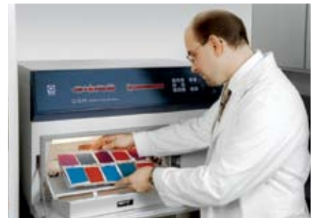
Easily mount parts, bottles, test tubes and petri dishes with the Q-Sun's unique slide out specimen tray.
